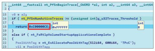
Figure 21: The nt!PfSnBeginTrace function returns prematurely if nt!PfSnNumActiveTraces surpasses the g\_u32Traces\_Threshold value.
