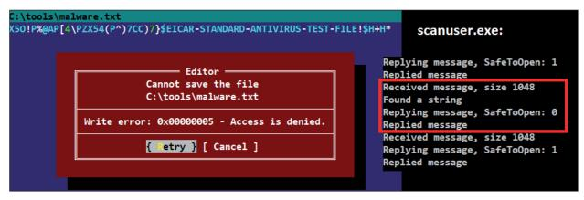
Figure 13: Write access to a file is denied when it contains a forbidden string.
