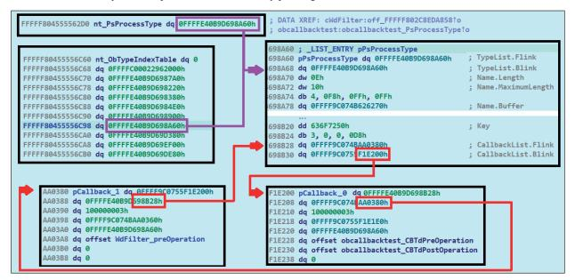
Figure 9. PsProcessType, one of the OBJECT\_TYPE structures in nt!ObTypeIndexTable. Highlighted in red is one direction of the doubly linked list containing two callbacks, for WdFilter.sys and ObCallBackTest.sys.
