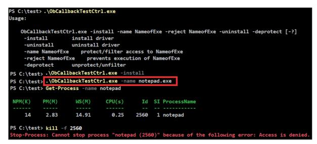
Figure 7: It's not possible to kill notepad.exe after registering an object callback that controls process creation.
