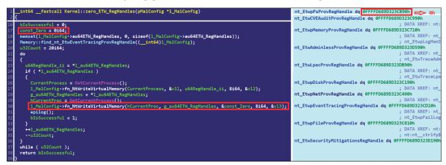
Figure 19: On the left, FudModule's implementation. On the right, its effect of zeroing all ETW Register Handles during runtime, with only one provider highlighted in red.
