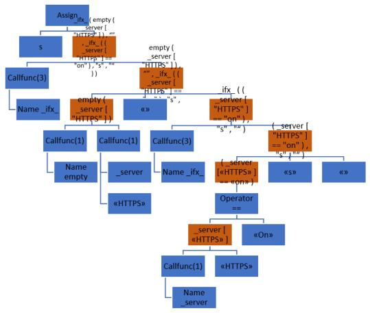
Like the first example, we split the line left and right from the assign. As long as we don't have an atomic result (orange) we keep on performing the process again and again until each node is an atomic element. Have a look at the more table-driven version of the same tree:
