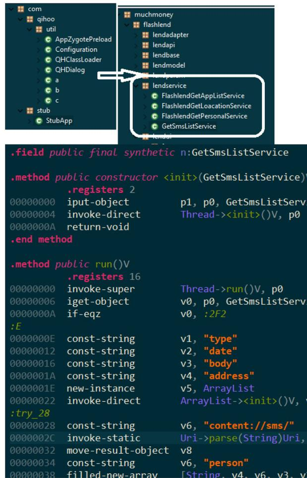
Figure 28: Jiagu packed vs unpacked.
