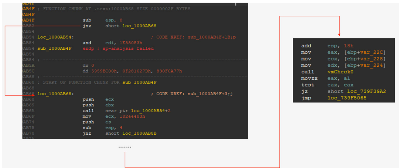
Figure 23: Control flow obfuscation using jcc opcodes.
