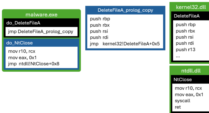
Figure 28: Illustration of code splicing kernel32.dll and ntdll.dll functions.
