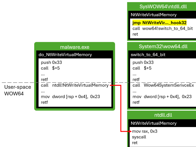
Figure 18: Illustration of Heaven's Gate skip WOW64 layer variant.
