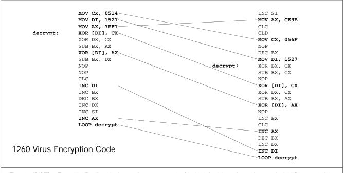
Figure 1: 1260 Virus Encryption Routine: This diagram shows two examples of the 1260 virus' decryption routine. Note that both files contain eight of the same instructions - these set up the encryption loop. The other instructions are chosen at random, in such a way that they do not affect the contents of the registers used for the decryption routine. This makes the virus impossible to find using a simple hexadecimal pattern search.
