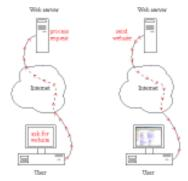
Figure 1: Normal HTTP traffic handling.
