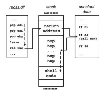
Figure 1: Memory layout and control flow.
