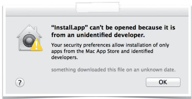
Figure 16: With the quarantine attribute set, Gatekeeper displays an alert.
