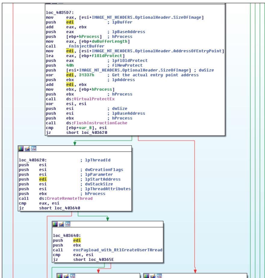
Figure 2: Remote code execution using `CreateRemoteThread`/`RtlCreateUserThread`.
