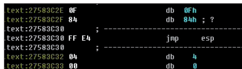
Figure 4: Jmp esp instruction in MSCOMCTL.OCX (v6.01.9545).
