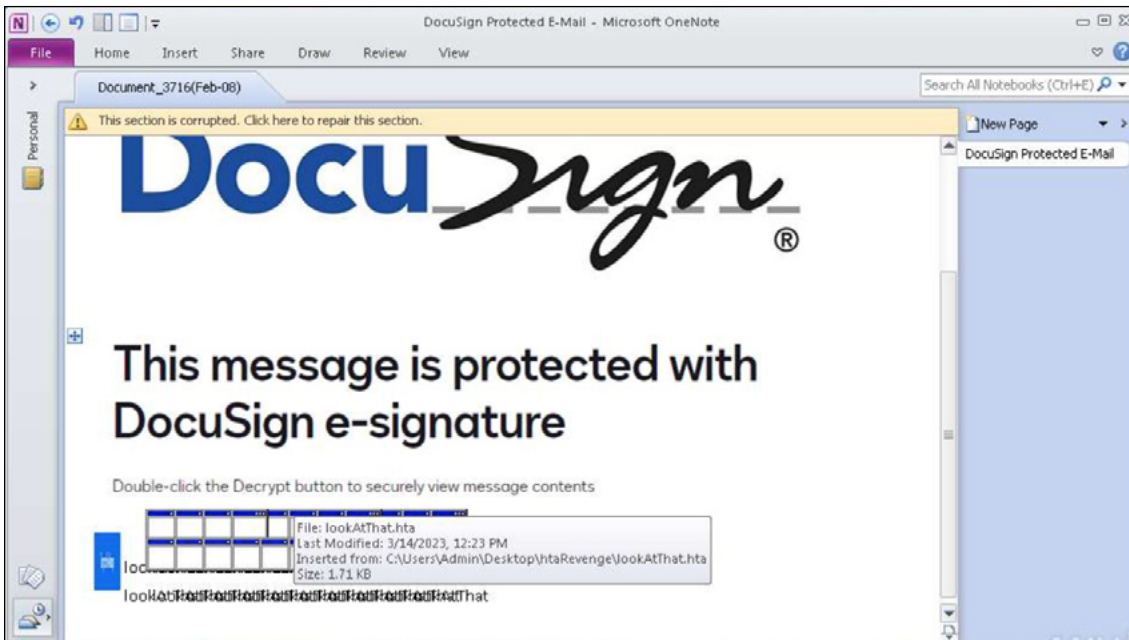
OneNote file with the .hta files hidden under an overlaid image resembling a button.
